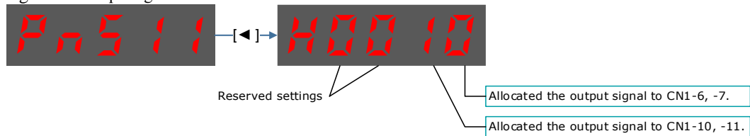
Figure 6-3 Output signals allocated
